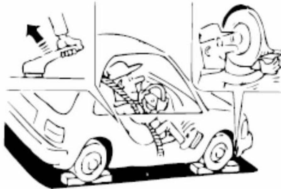
Start the engine, depress the brake pedal, and turn the shift lever to D position.
